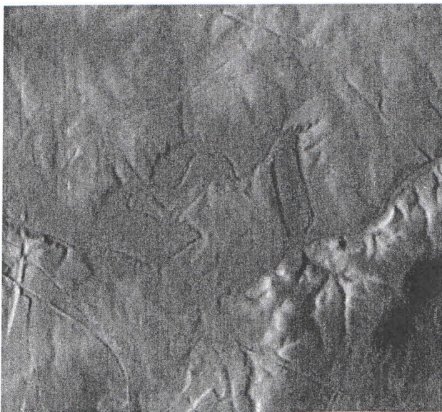
Figure 5 – Digital elevation model (DEM) obtained by LIDAR (source: http://web.cs.swarthmore.edu )
