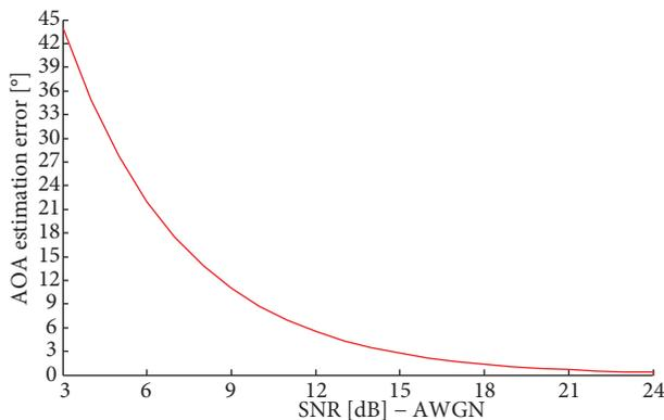
**Figure 7.** AOA estimation error [°] versus SNR [dB].
