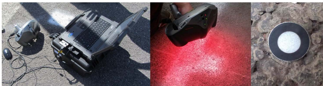
Obr.3. 3D Zscanner 800 – MPD, R_a , R_q , priebeh skenovania, reflexný bod (Targets)
