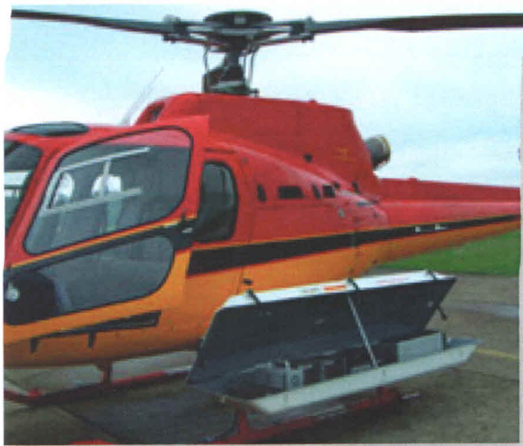
Figure 6: Mapping system installed on a helicopter.
